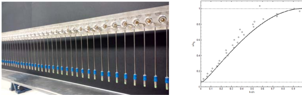
Figure 1. Left - Picture of the experimental chain of magnets. Right - Theoretical (continuous line) and experimentally measured (dots) dispersion of the chain
